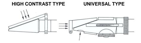
**REMARK**: Only for the RF.5190, a special daylight window for untransparent specimens is provided. Usually it should be kept closed.
